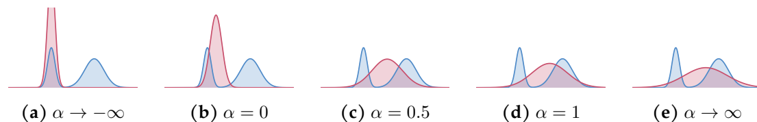
Figure 2.4: Overlay of a bimodal target density p(\theta) (blue) and its variational approximation q(\theta) (red) for five divergence parameters \alpha . Each panel shows both densities with semi-transparent fills to emphasize the probability mass. The sequence from left to right demonstrates the transition from extreme mode-seeking ( \alpha \rightarrow -\infty ) through the reverse-KL ( \alpha = 0 ), an intermediate trade-off ( \alpha = 0.5 ), the forward-KL ( \alpha = 1 ), to strong mass-covering behavior ( \alpha \rightarrow \infty ).
